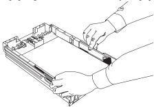
3. If necessary, lift and adjust the vertical paper guide for the length of your paper.
